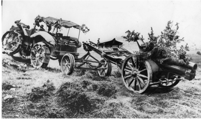
An elderly 149/13 howitzer being towed by old Pavesi tractor in pre-war maneuvers. By the time war broke out the dolly wheel supporting the trails had usually been replaced by a trailer that carried the gun, permitting slightly higher speeds.
